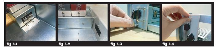
Gently slide the MODULE onto the RACK TRAY making sure the MODULE glides over the GUIDE BRACKETS smoothly without restriction, as illustrated in fig 4.1. Adjusting the GUIDE BRACKETS may be necessary to line up the MODULE as it travels down the tray, make sure they are as centered and square as possible. Also Insure that the Cinch Jones Plug and Socket line up, as illustrated in fig 4.2.
